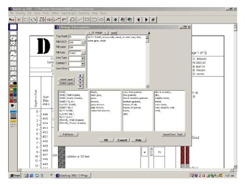
To speed entering soil and rock descriptions, you may set-up lists of often used description phrases (ex. "SAND, Poorly Graded," "yellowish brown," "traces of silt," etc). Then, you simply click on these phrases to have them placed in the description text box, above. Also, you can use this method to standardize description entry so that your logs become more consistent.
