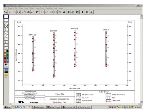
In addition to labeling the layers, you may choose to have them filled with a fill pattern inside the representation of the borehole:
